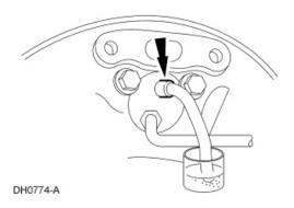
Brake System — General Information - Brake System Bleeding - General Procedures • 2009 Ford Escape Hybrid • MotoLogic
