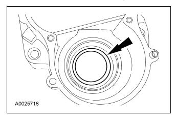
6. CAUTION: The transfer case cover and case sealing surfaces must be free of grease prior to applying new silicone sealant.
