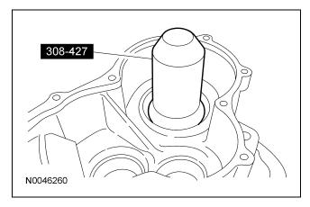
2. CAUTION: Take care not to roll the transfer case inner halfshaft seal lip when installing the drive gear.
