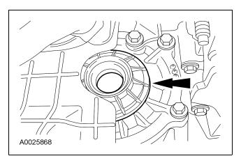
4. CAUTION: The transfer case cover is aligned with the case using 2 hollow dowels. Remove the cover squarely from the dowels to avoid cracking the cover bosses.
