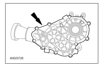
5. Remove the transfer case driven gear seal.
