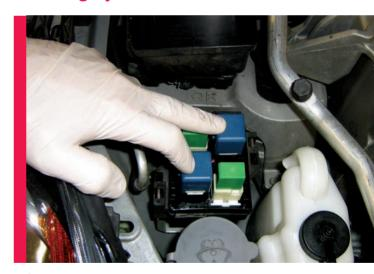
These are the ABS Pump Motor Relays.
