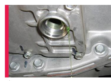
This is the inverter coolant drain in the transaxle. The other drain is on the inverter radiatior.
