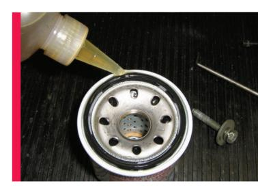
Always lubricate the oil filter gasket with clean motor oil so it won't become stuck in place. The "next guy" may be you!
