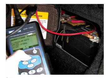
Test the 12V glass mat battery using an internal resistance tester such as the Midtronics EXP-1000 or EXP-1200.
