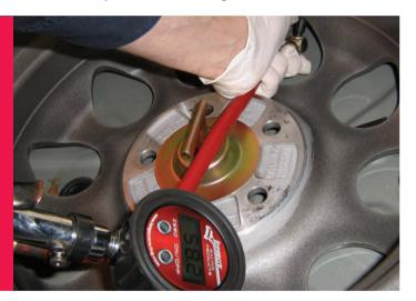
Check and fill the Altima Hybrid spare tire pressure to 60 psi.
