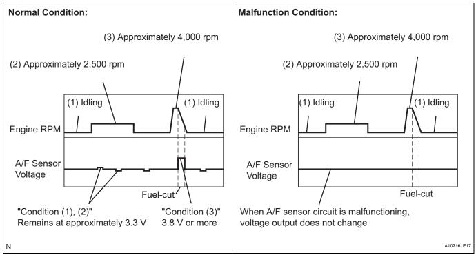
If the output voltage of the A/F sensor remains at approximately 3.3 V (see Malfunction Condition diagram) under any conditions, including those above, the A/F sensor may have an open circuit. (This will also happen if the A/F sensor heater has an open circuit.)
