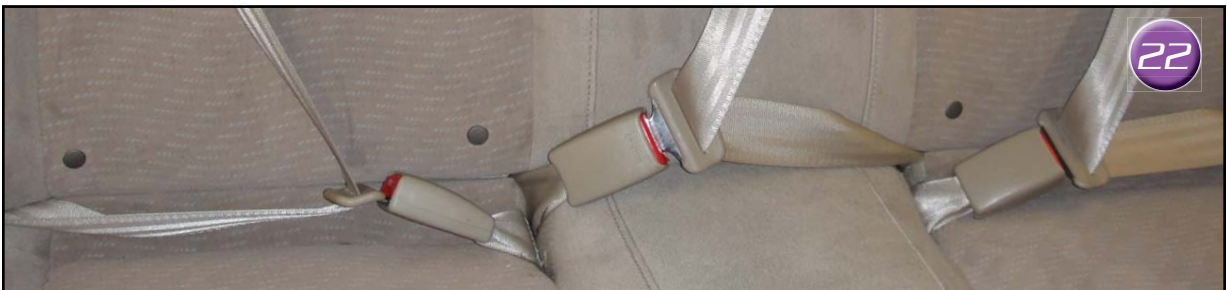
Often overlooked- Connect all of the seat belts to make sure none are still stuck under the seat or twisted any time the seat was removed.
