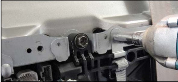
The IMA battery module is held in place with four bolts and one retaining bracket.
