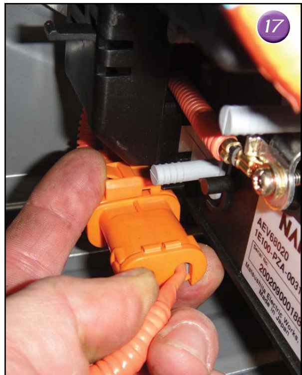
This connector must be removed from its mount before it can be separated
