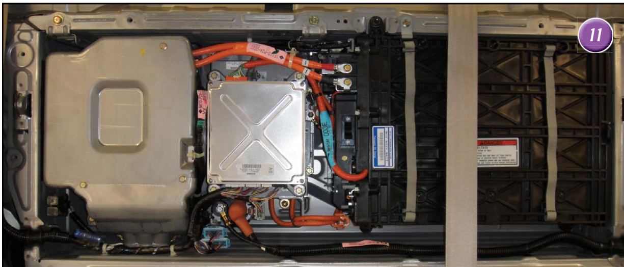
IMA battery is a black box with two straps on the right.
